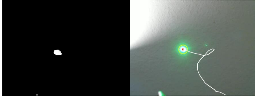
Left: Filtered input indicating which pixels fall within set HSV/HSL parameters Right: Input frame overlaid with detection indicator and track of object movement
