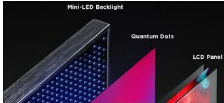
Figure 28: How LED work in a monitor [42]
