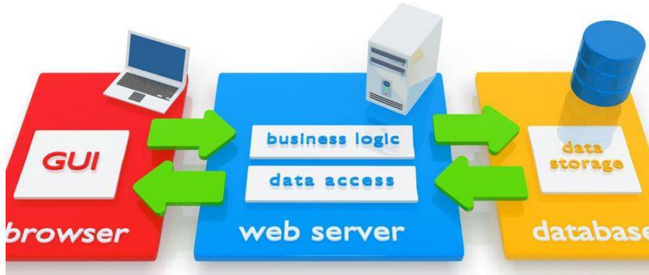
Figure 9: Graphical flow diagram of a web-based application [5]
