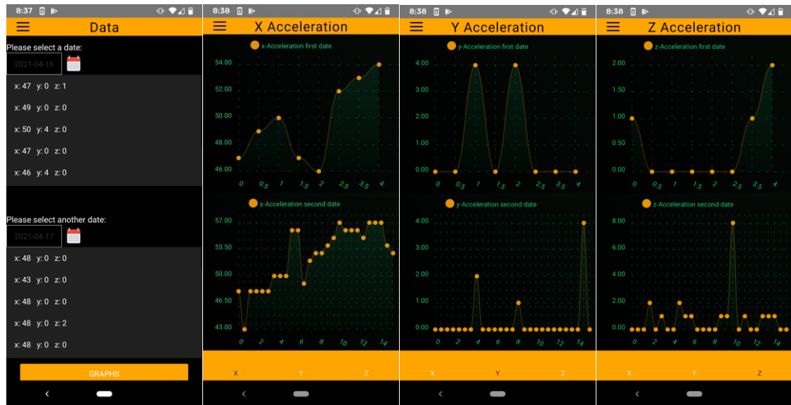
Figure 31: UI for Data Display. Above showcases the Data Screen, where a user can select two dates to compare the accelerometer data of those two dates. The remaining screens demonstrate the individual acceleration Tab Screens, where the data for each date correspond to a singular graph on each screen.
