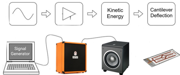
Fig. 2. A signal is generated (left), amplified through a bass guitar amplifier, the amplified signal is sent to a subwoofer, and the subwoofer vibrates the cantilever (right).
