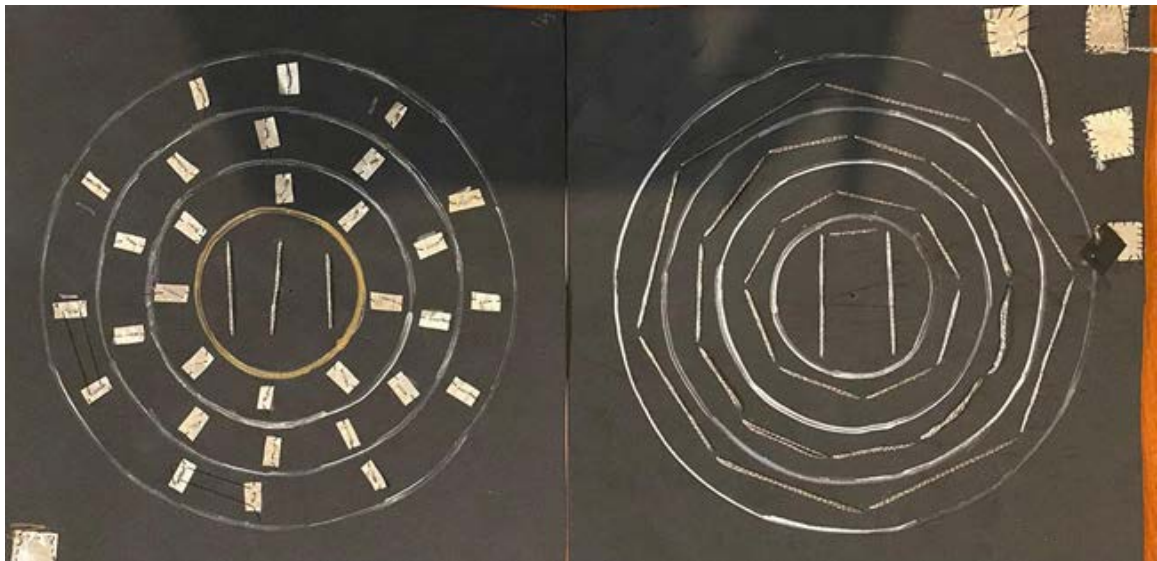
Figure 15: Side B Sensor Target Internals: (left) Voltage area for the pressure sensor.(right) Side B area divided between four areas for demarking the accurate areas.
