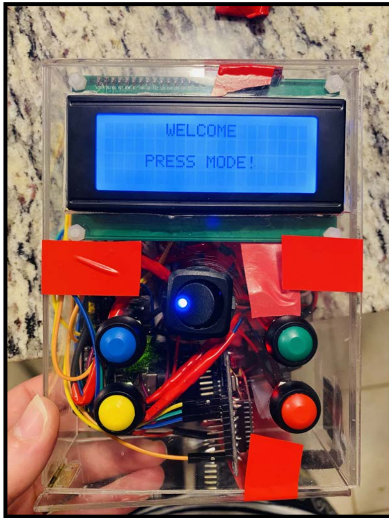
Figure 25 (top): Physical Implementation of Remote Case, Side View
