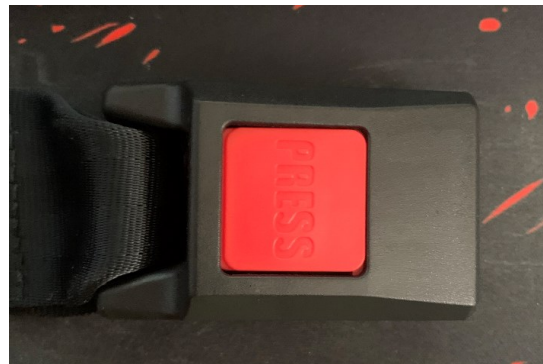
Figure 46: Side Release Lock Assembly
