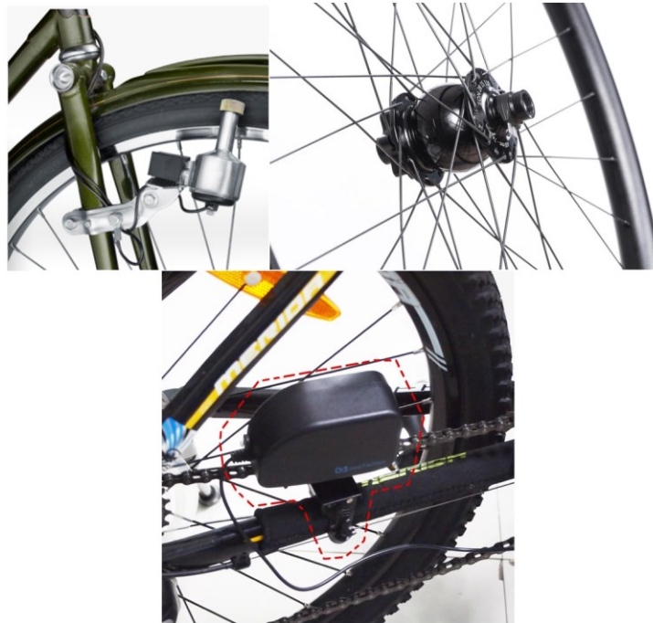
Figure 27: Different Bike Dynamo Configurations to Generate Power [7][8][9]
