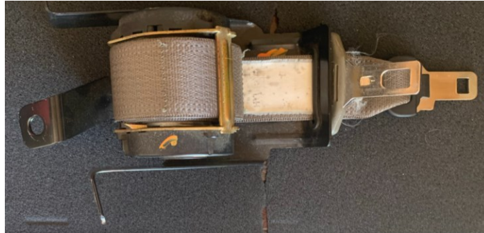
Figure 44: Inertial Reel Assembly
