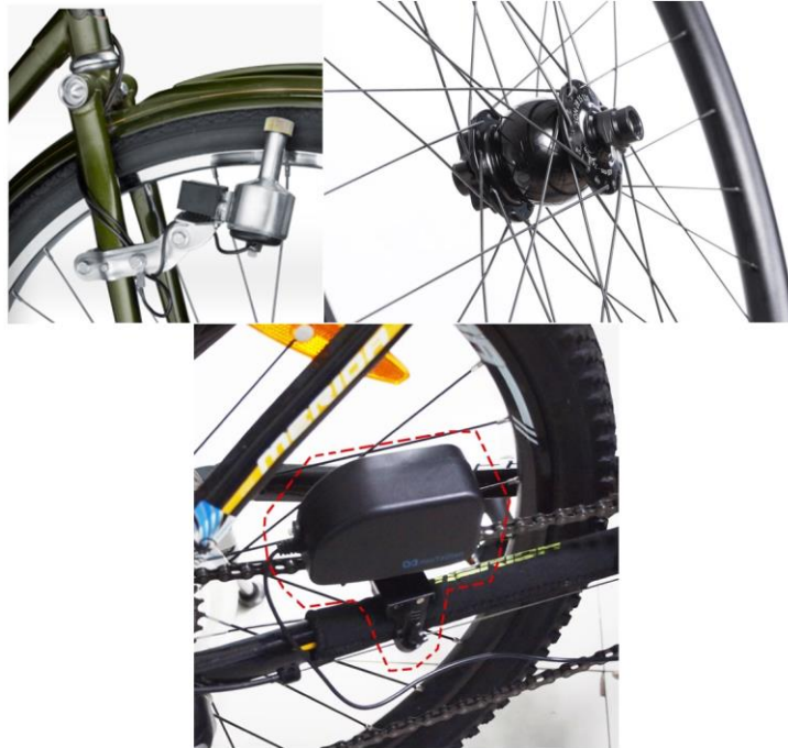
Figure 27: Different Bike Dynamo Configurations to Generate Power [7][8][9]
