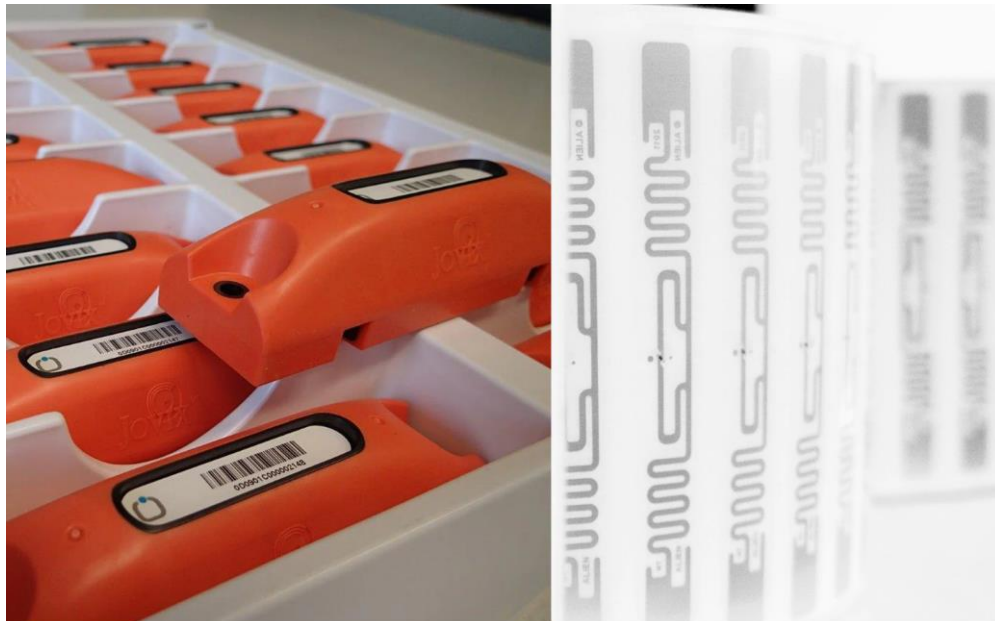
Figure 19: An example of an active tag (left) versus a passive tag (right)
