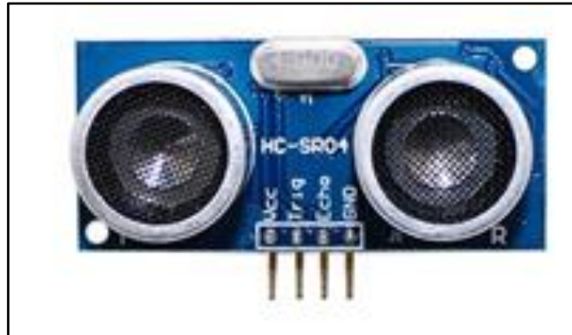
Figure 31 - Cuisimax HC-SR04 Ultrasonic Sensor Distance Measuring Module
