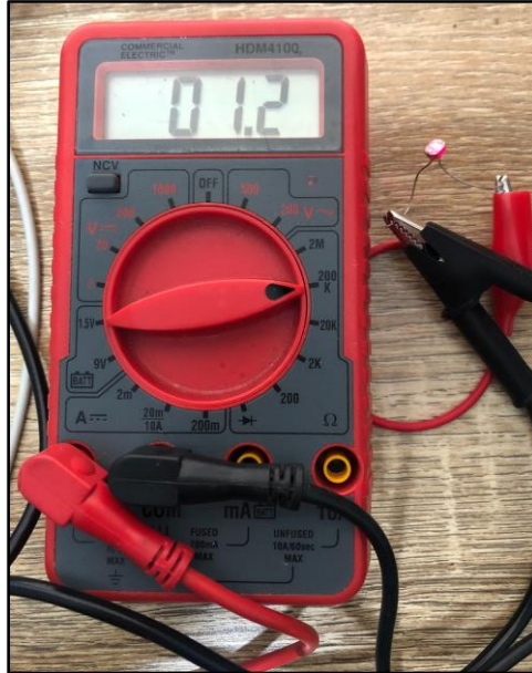
Figure 80 - Using Laser Diode as Light Source Measuring Resistance
