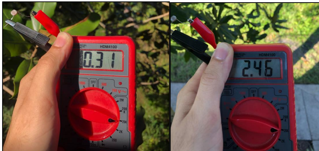
Figure 82 - Outside LDR Testing in Direct and Indirect Sunlight
