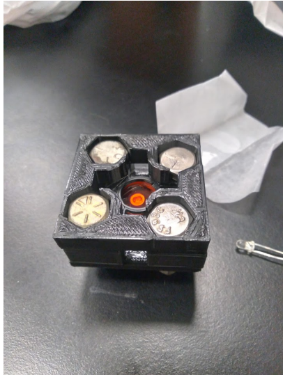
Figure 53: 3d-printed optode housing, containing LEDs, photodiode and filter
