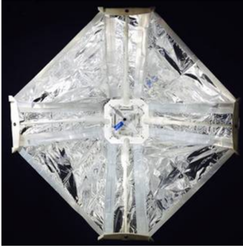
End view of Sunshield on CryoCube-1 developed at Sierra Lobo. Credits: Sierra Lobo (2014).
