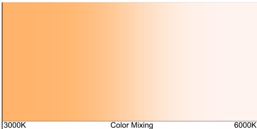
Figure 9 : An example of possible light color temperatures available by modulating the power of the two LED strips.
