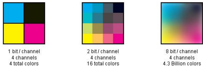
Figure 7: Color bit depth, As the number of color bits increases, the total possible colors mixable increases exponentially.
