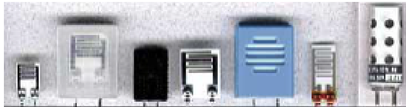
Figure 19: Variations of resistive humidity sensors [Fierce Electronics]
