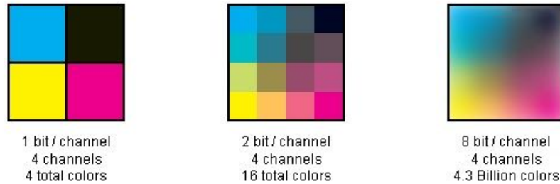
Figure 9: Color bit depth, As the number of color bits increases, the total possible colors mixable increases exponentially.
