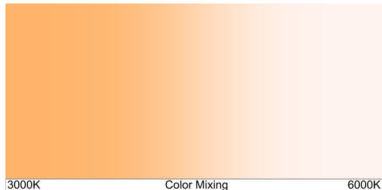
Figure 11 : An example of possible light color temperatures available by modulating the power of the two LED strips.
