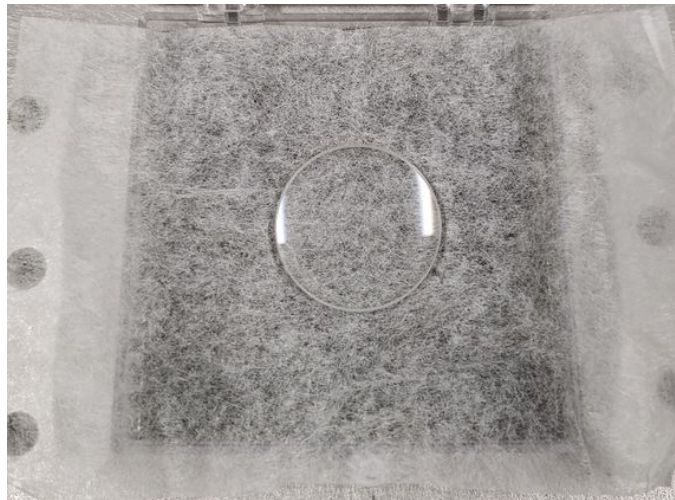
Fig. 67: Newport KBX061 bi-convex uncoated lens for collimating the Raman output. No laser induced damage on its surface and good transmission up to 2000nm wavelength.
