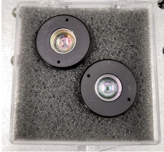
Fig. 68: Pair of Thorlabs A240TM-C lenses without any visible laser damage that would impact their performance.
