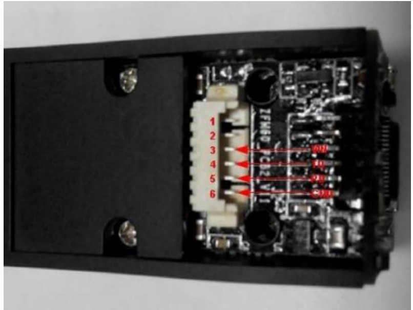
Figure 38: SEN0188 connection pins
