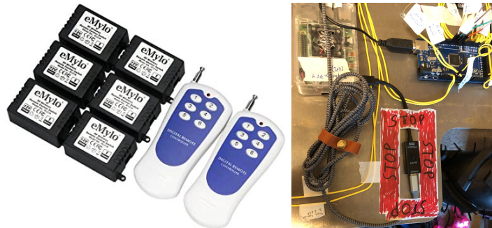
Figure 9.1.4-1: Remote and Physical Emergency Stops
