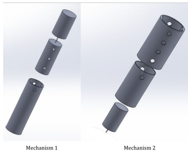
Figure 6.2.3-1: Initial Adjustable Height Mechanism Designs
