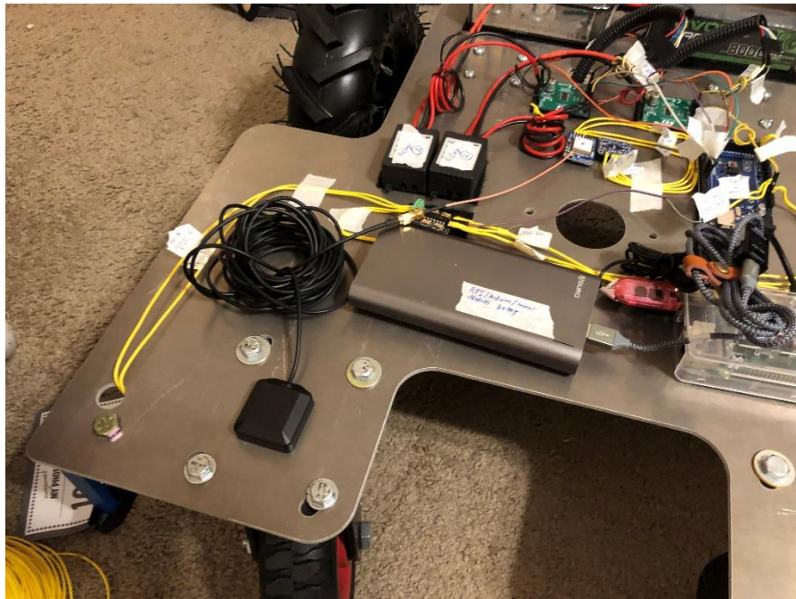
Figure 46: Integrated GPS Module and Antenna on Rover
