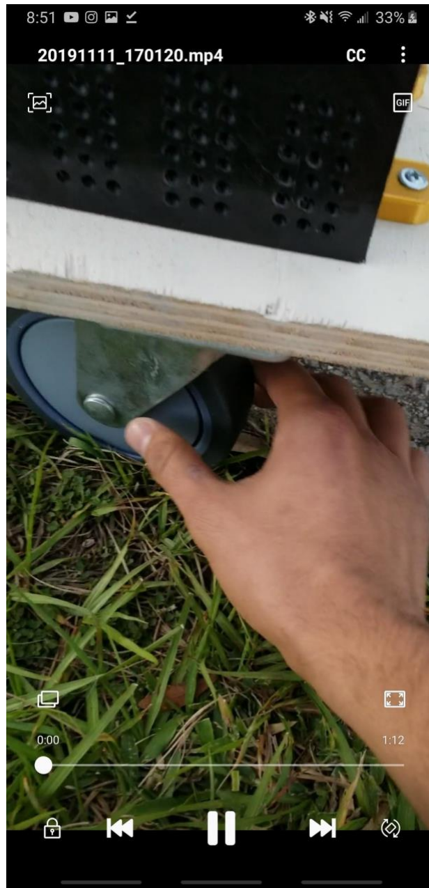
Figure 71: alphagoat getting stuck because swivel wheel
