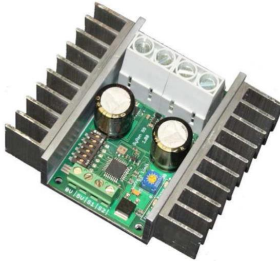
Figure 38: Syren 50A Motor Controller
