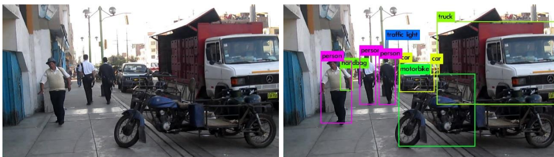
Figure 7, base image passed to and predictor image returned from the YOLOv3 trained model
