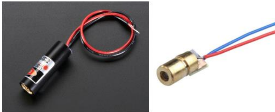
Figure 11 Adafruit (left) and HiLetgo (right) Red Laser Diodes Permissions in Figure 26 and Figure 27
