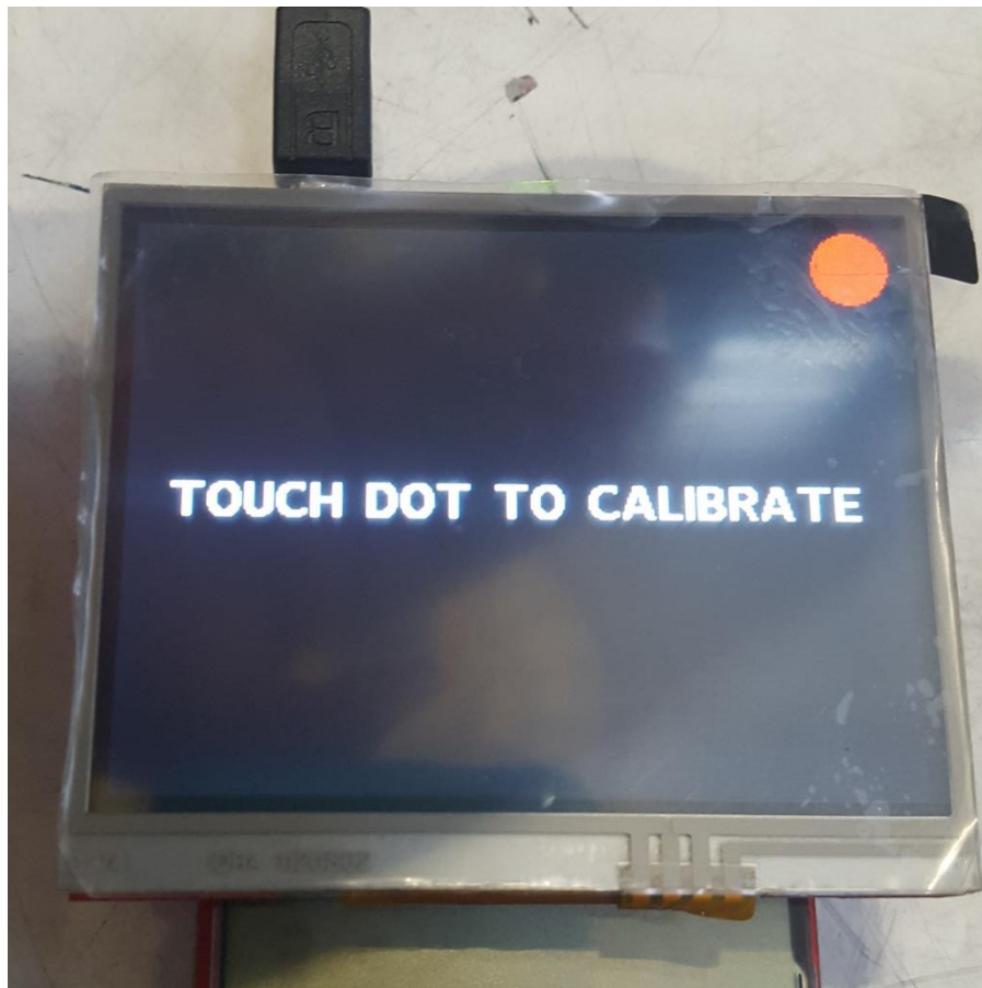
Figure 53. Calibration of screen for touchscreen.
