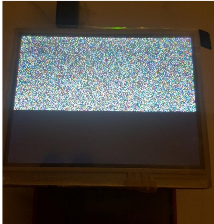
Figure 51. Display being reset using command over SPI.
