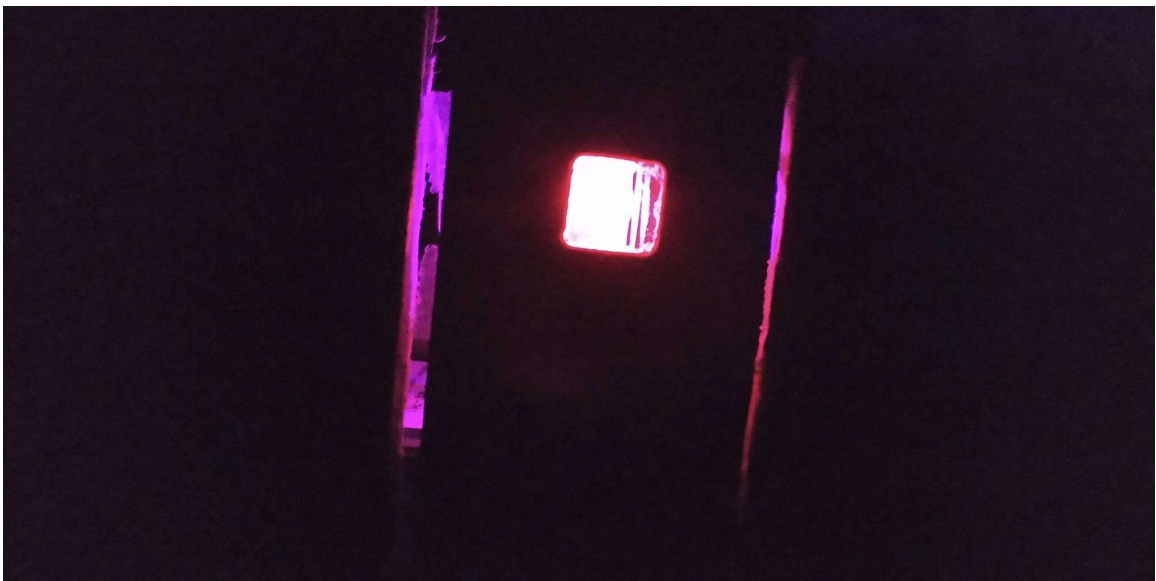
Figure 53. Fluorescent light at the collimating mirror interface through the longpass filter
