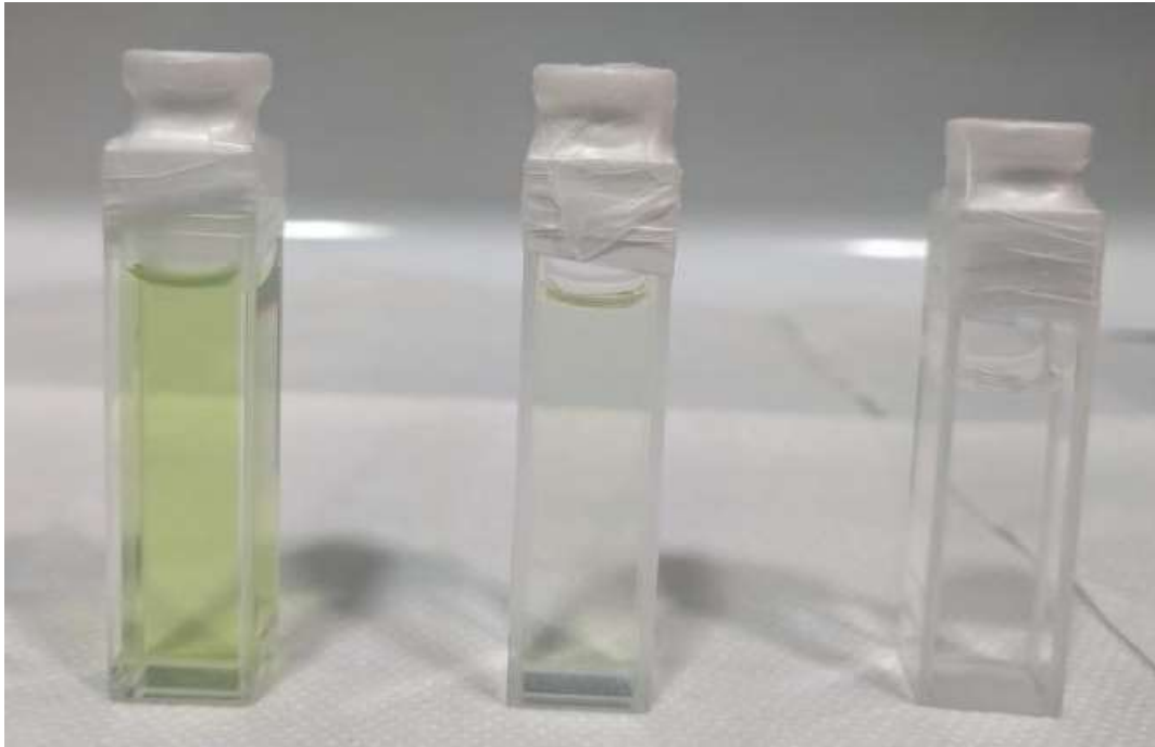
Figure 9. From left to right: Chlorophyll a sample diluted with 150mL (high concentration), Chlorophyll a sample after diluted until OD < 0.1 , pure acetone.
