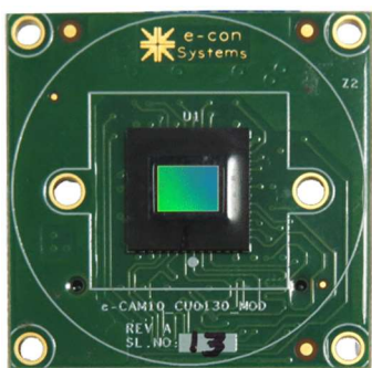
Figure 11. AR0130CS (ARDR) imaging sensor on a PCB
