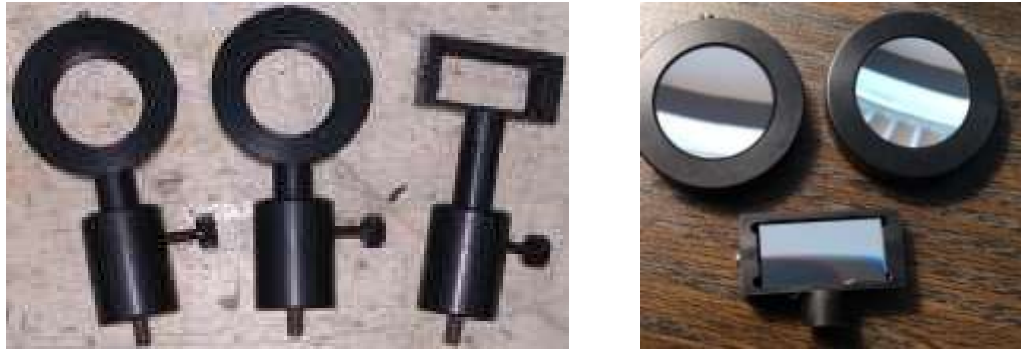
Figure 57. Empty posts and holders (left); optics mounted in holders (right)
