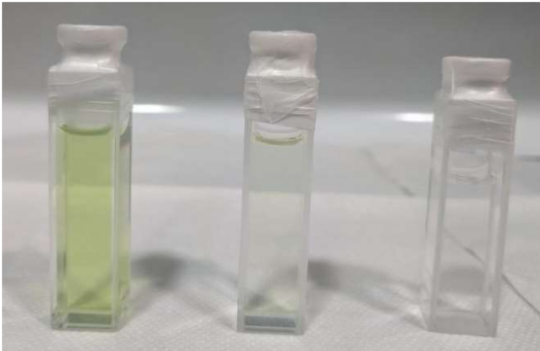
Figure 12. From left to right: Chlorophyll a sample diluted with 150mL (high concentration), Chlorophyll a sample after diluted until OD < 0.1 , pure acetone.
