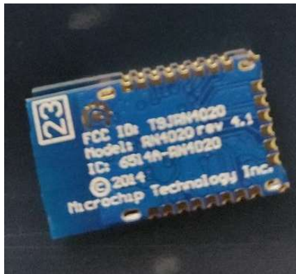
Figure 51. RN4020 Bluetooth Module
