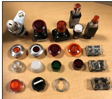
Figure 34: Allen-Bradley Control Panel Parts
