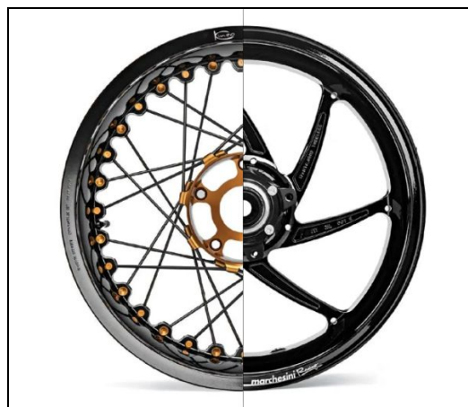
Figure 43: Spoked Wheel (left) Alloy Wheel (right)
