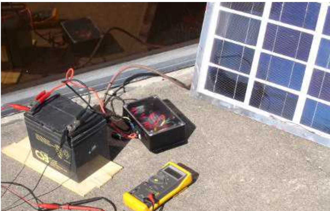
Figure 40. Charge Controller Testing Setup with Solar Panel
