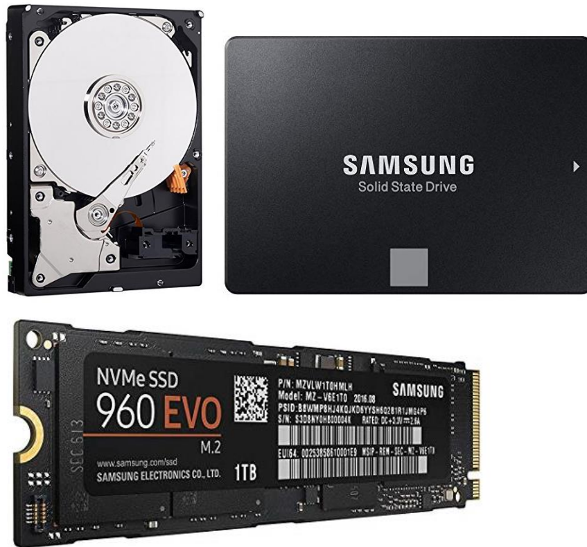
Figure 3.5.2.1(a)(b)(c): Top left: magnetic disk drive (25). Top right: SATA SSD (26). Bottom: M.2 PCIe SSD (27)
