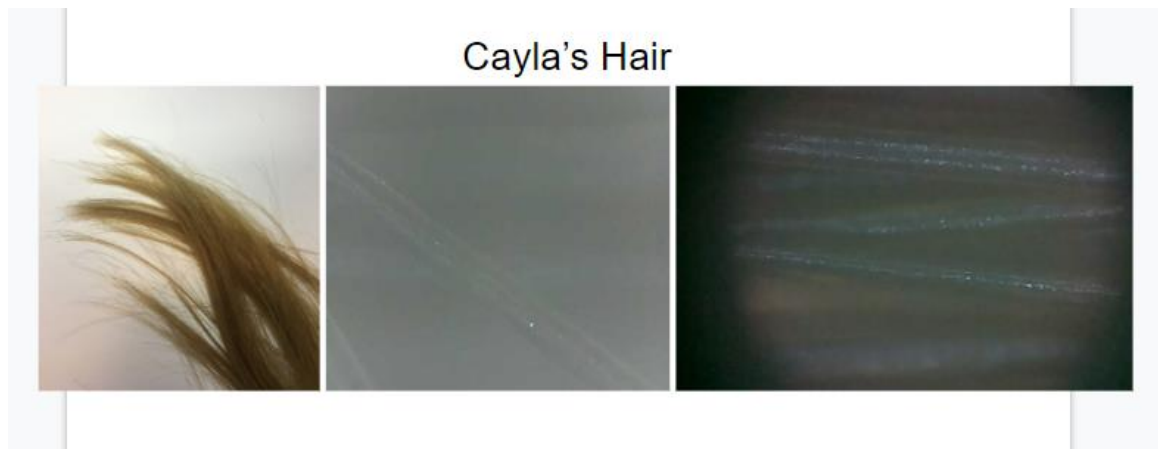
Figure 75: Cayla's Hair Aperture Testing- Shows the increase in both resolution and contrast.
