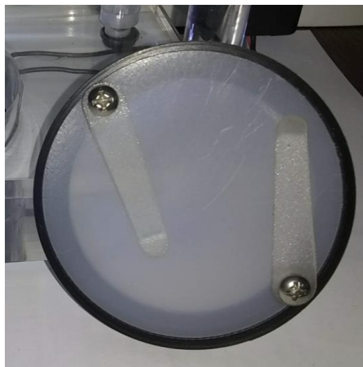
Figure 20: Diffusion Filter with Clips
