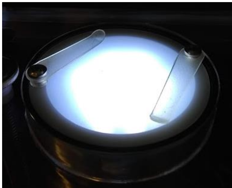
Figure 29 Even Distribution of Light using Diffusion Filter
