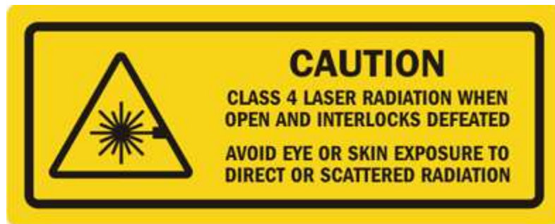
Figure 12: Example of a class 4 laser safety label (MySafetyLabels).
