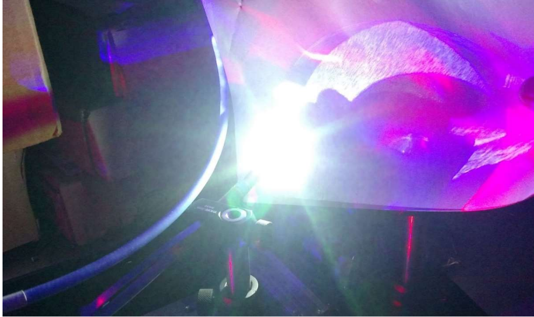
Photo 5: First time achieving white light from a single multimode fiber
