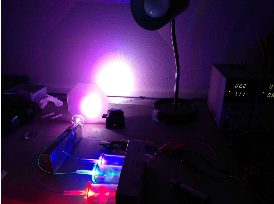
Photo 7: Achieving speckle-free white light from fiber-coupled laser diodes
