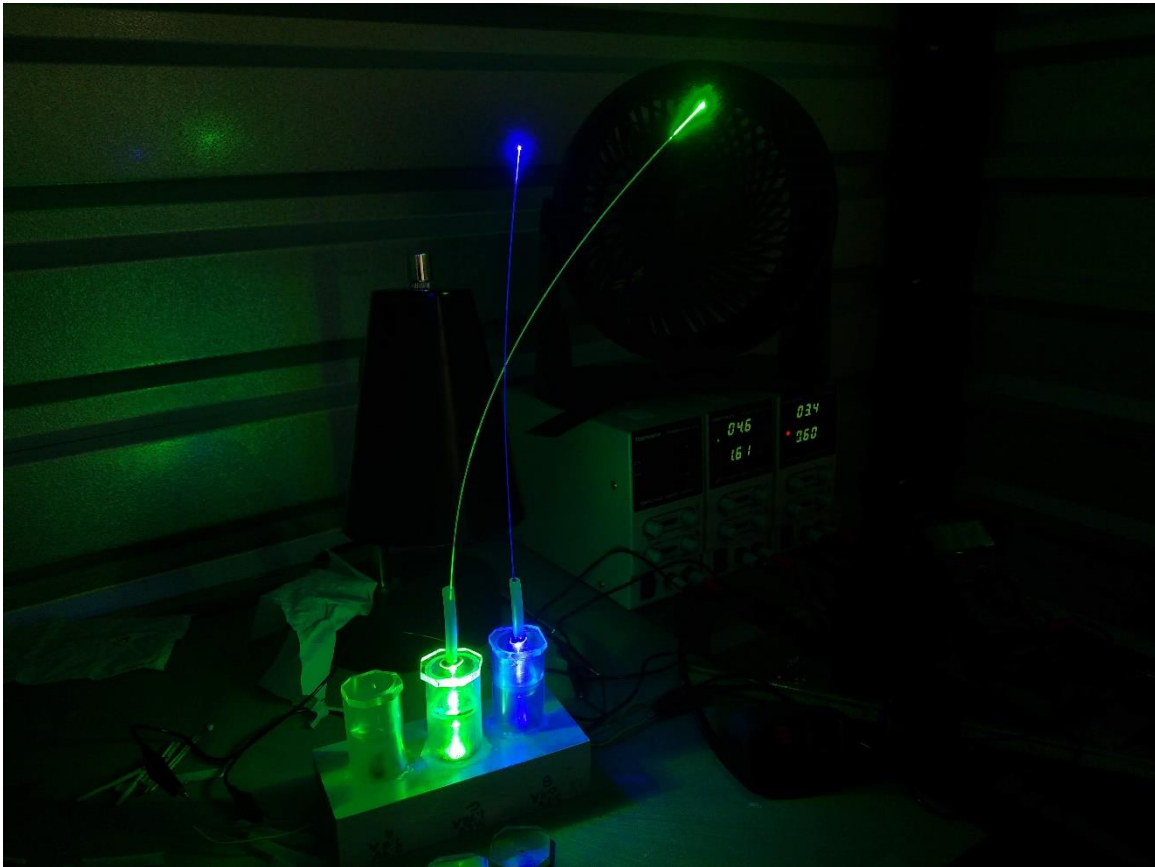
Figure 53: Initial Testing of the Multi-Tube Diode-Fiber Coupling Method
