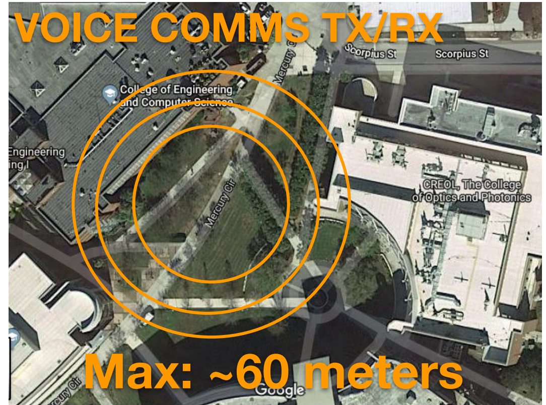
NRF24LO1+ TRANSCEIVER VOICE COMMUNICATIONS RANGE TEST
