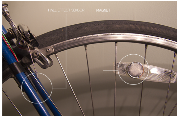
Figure 10. Hall Effect Sensor Placement
