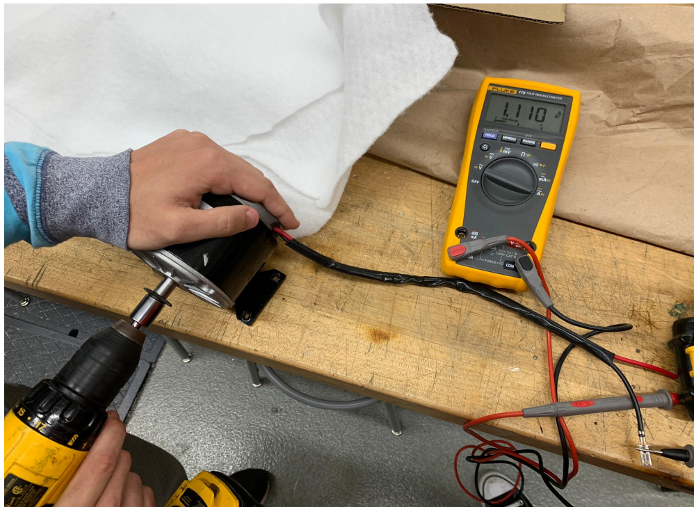
Figure 72. Amp Output of DC Generator
