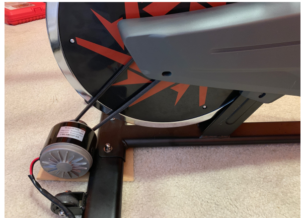
Fig. 1. Setup of motor generator
