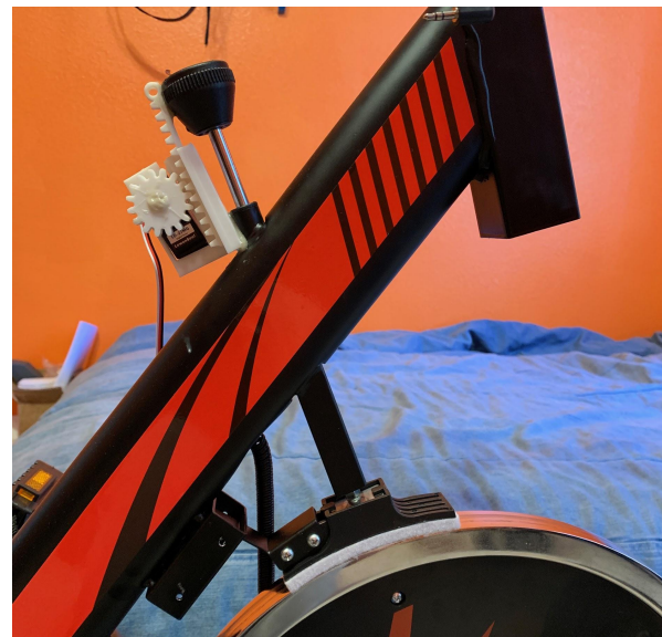
Fig 3. Bicycle resistance system attached to stationary bicycle.
