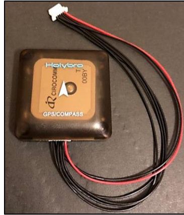
Figure 29: Holybro Micro M8N GPS Module picture taken by Brandei Dieter
