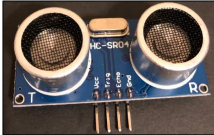
Figure 27: HC-SR04 Ultrasonic Sensor picture taken by Brandei Dieter
