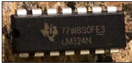
Figure 23: LM324N Operational Amplifier picture taken by Brandei Dieter
