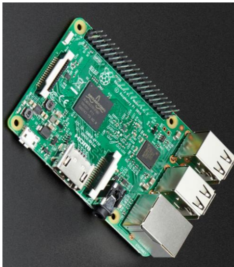
Figure 16: Raspberry Pi Model 3 B used with permission from Adafruit.com [32]
