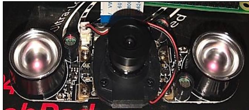
Figure 23: Raspberry Pi 3 Model B Night Vision Camera picture taken by Brandei Dieter
