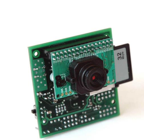
Figure 10. A Camera and sensors can be added for more robust bolt to bolt and socket to nut alignment using edge detection software
