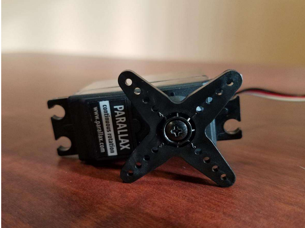
Figure: Acquired Gearmotor 6 V DC Servo
