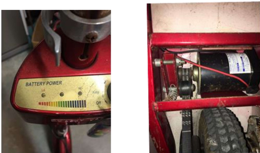
Figures: Battery Powered Scooter Battery Indicator (left) and Drive Train (right)
