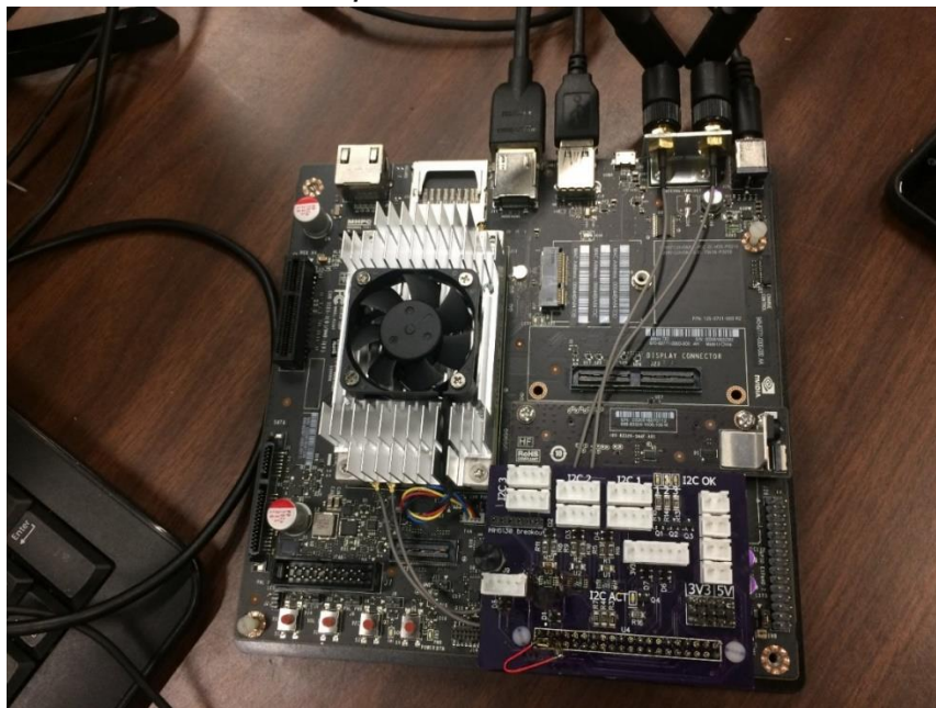
Figure 9. NVIDIA Jetson close-up with I2C isolation PCB mounted
