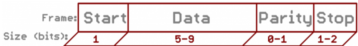
Figure 25. A frame of asynchronous serial data (Sparkfun Electronics, 2012). The use of this image is governed by the CC BY-SA 4.0 (Creative Commons Corporation, 2013).
