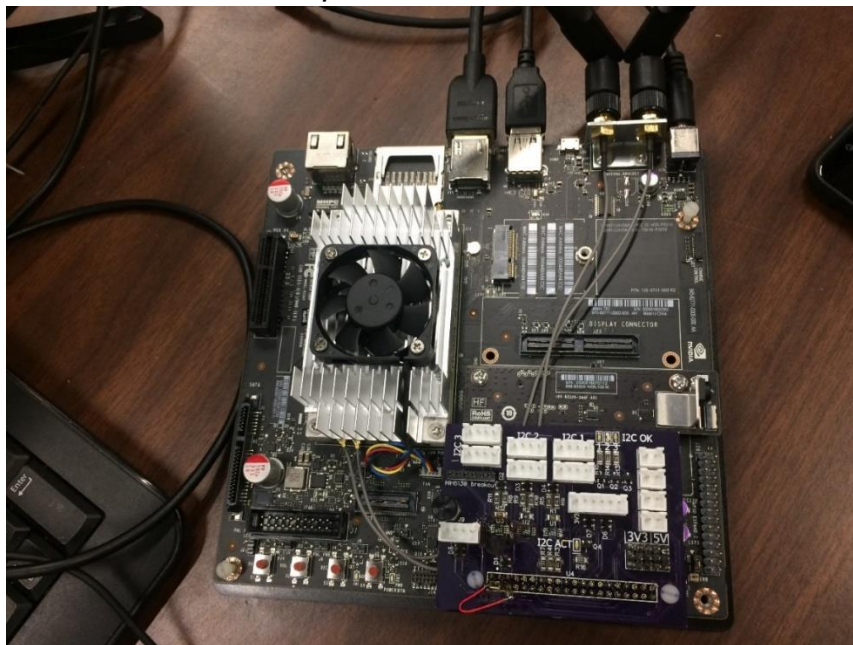
Figure 8. NVIDIA Jetson close-up with I2C isolation PCB mounted
