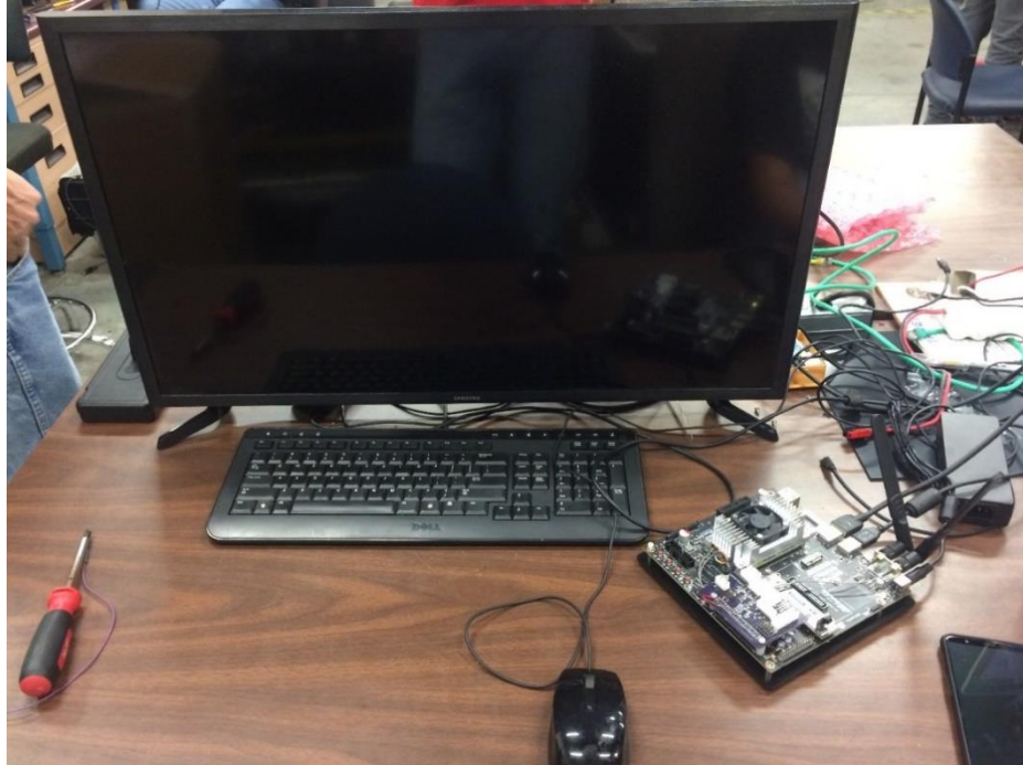
Figure 7. NVIDIA Jetson Dev Kit connected for testing
