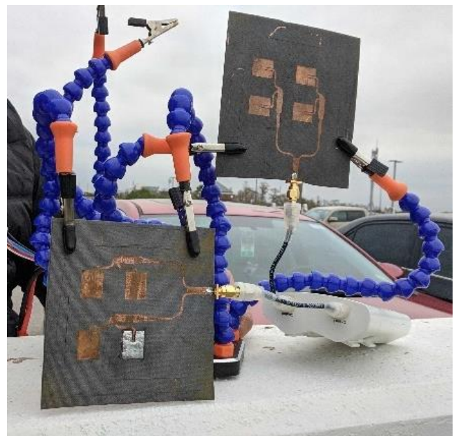
Fig. 3. Custom patch antennas connected to the Rocket M5 for range testing on the libra parking garage
