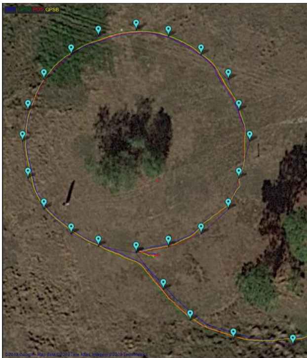
Fig. 8. Vehicle GPS track during waypoint test. Waypoints are in light blue and the vehicle track is in yellow.
