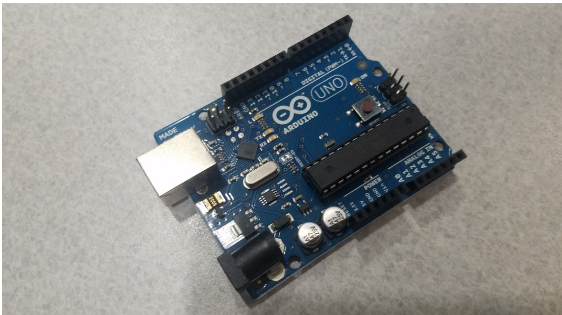
Figure 17: Arduino Uno R3
