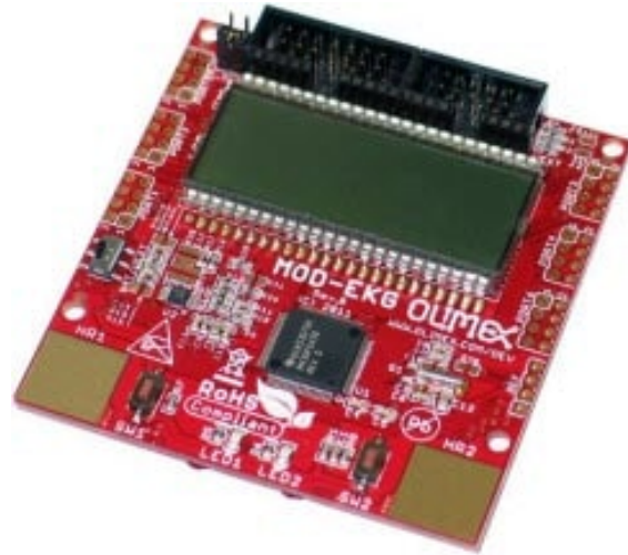
Figure 23: Olimex Medical Series Board
