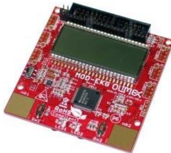
Figure 23: Olimex Medical Series Board
