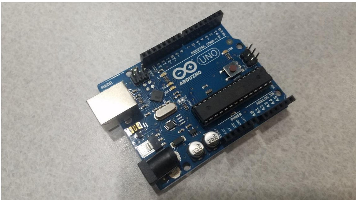
Figure 17: Arduino Uno R3
