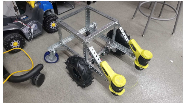
Figure 6: Early stage of eGOAT creation with trimmer motors and drive motors attached.
