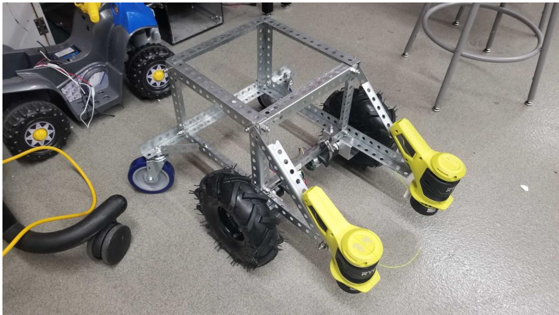
Figure 6.17 eGOAT first phase mechanical structure
