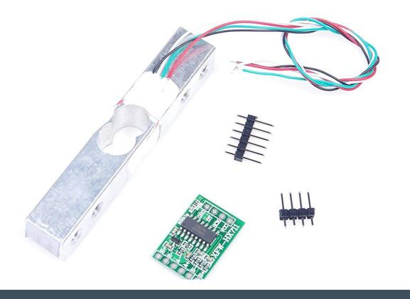
Digital Load Cell Weight Sensor
