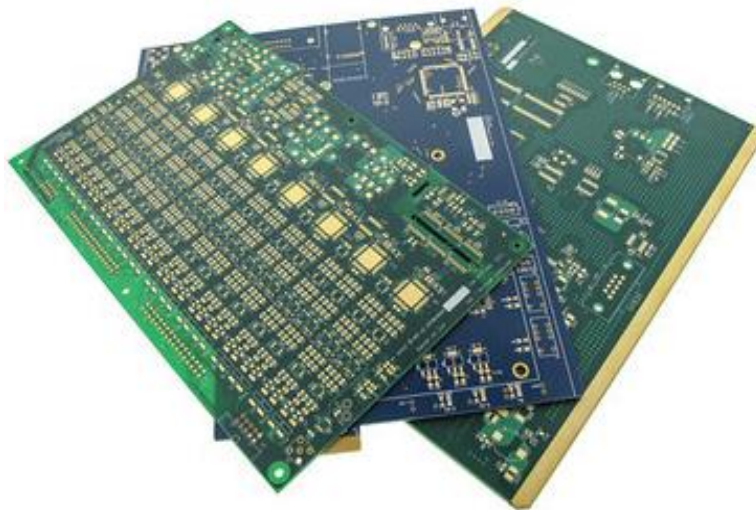
Figure 5: Multilayer Printed Circuit Board
