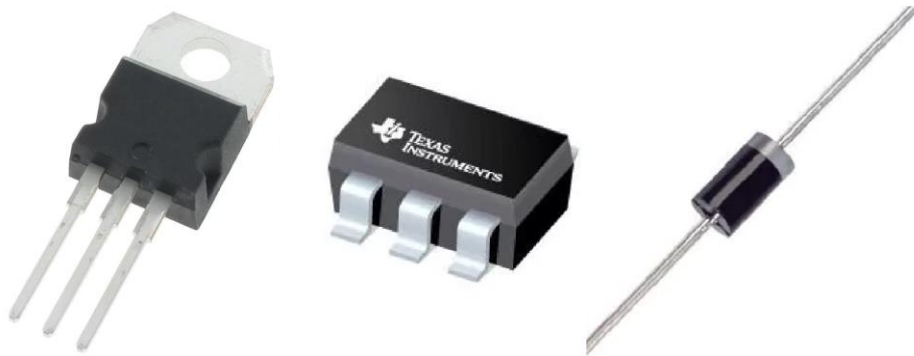
Figure 20: Linear, Switching, and Zener Diode Voltage Regulators
