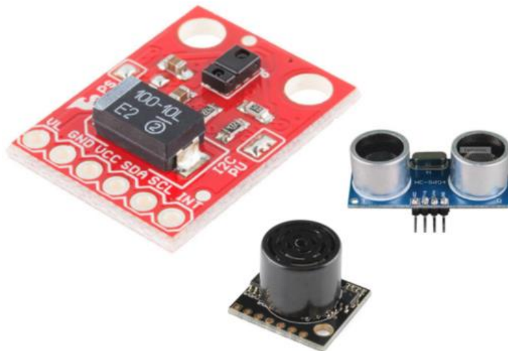
Figure 49: Ultrasonic Range Finder (bottom), HC-SR04 (top right), Gesture Sensor and RGB Finder (top left)
