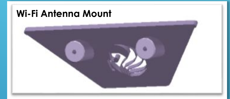
Designed to mount antenna – fixed to rear bumper
