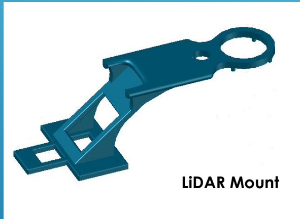
Designed for minimal vibration – fixed to Jetson Board
