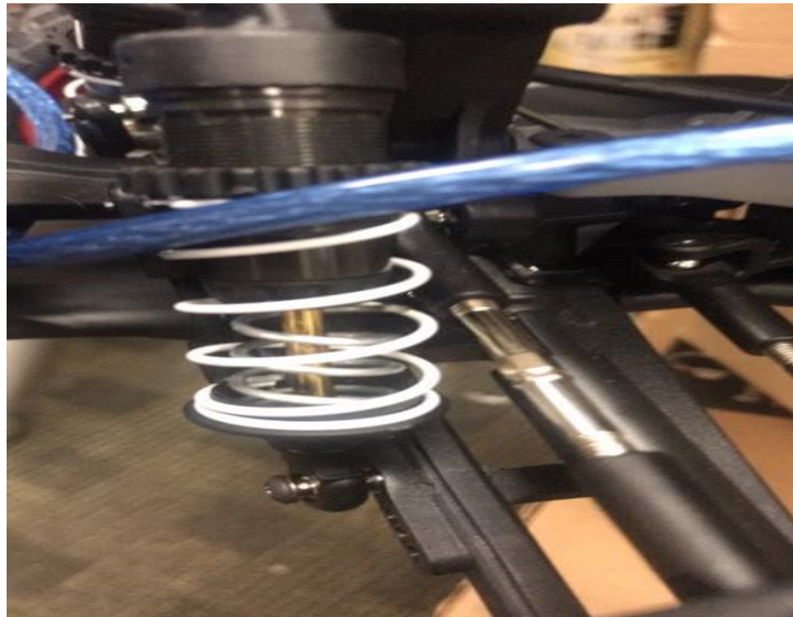
Figure 46- Two Springs in Parallel on the Shock
