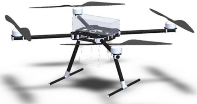
Fig. 2. CAD model of our drone fully assembled. The battery is shown mounted to the top of the frame, with the payload hanging below.
