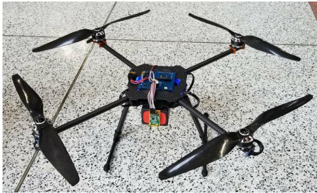
Fig. 1. Image of our microgravity drone almost fully assembled. The payload bay will hang below the frame, the mission computer will sit on the payload bay and the battery will be mounted on the top of the frame. This configuration was used to perform an initial flight to test the stabilization PID settings.
