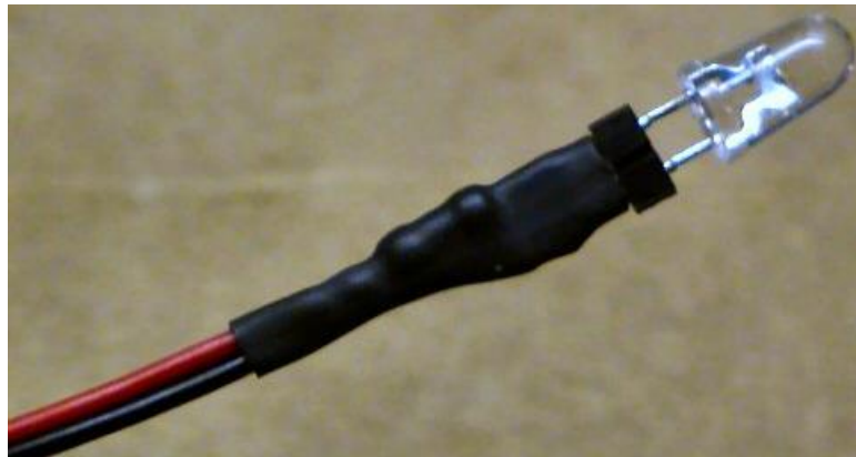
Figure 35 heat shrink over exposed leads (Permission Pending)
