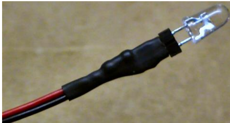
Figure 35 heat shrink over exposed leads (Permission Pending)
