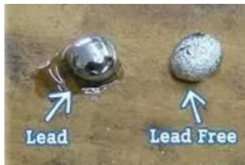
Figure 33 Balls of lead and leadfree paste (Permission Pending)
