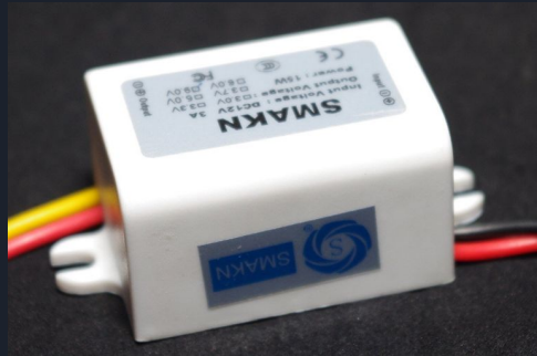
12V Step Down to 9V Power Supply
