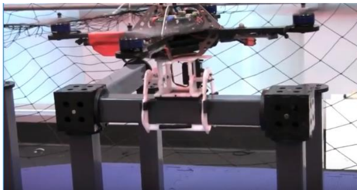
Figure 2: Autonomous Construction Quadrotor [3]
